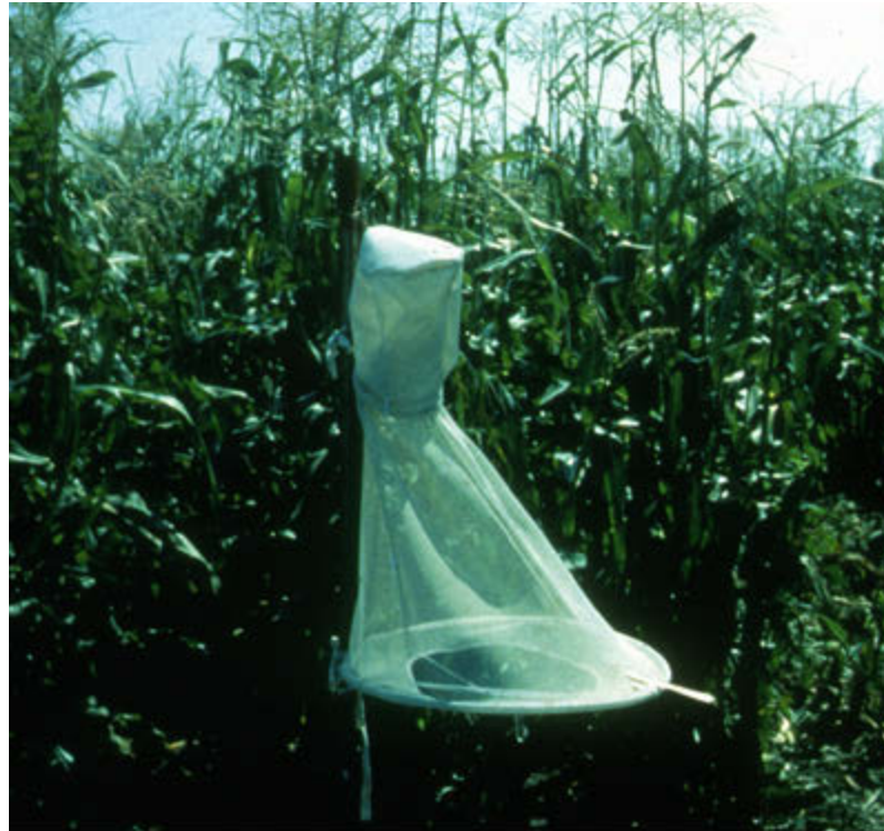
Hartstack corn earworm pheromone trap [ Picture by R. Foster ]
