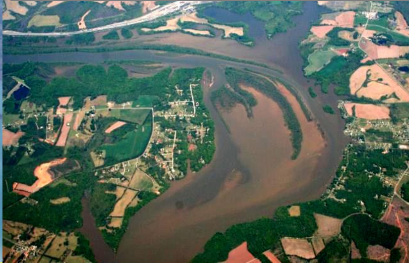
Erosion from bare fields into river
