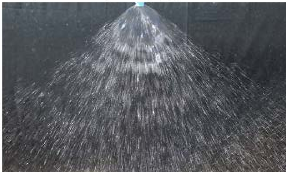
Example of an acceptable spray pattern
