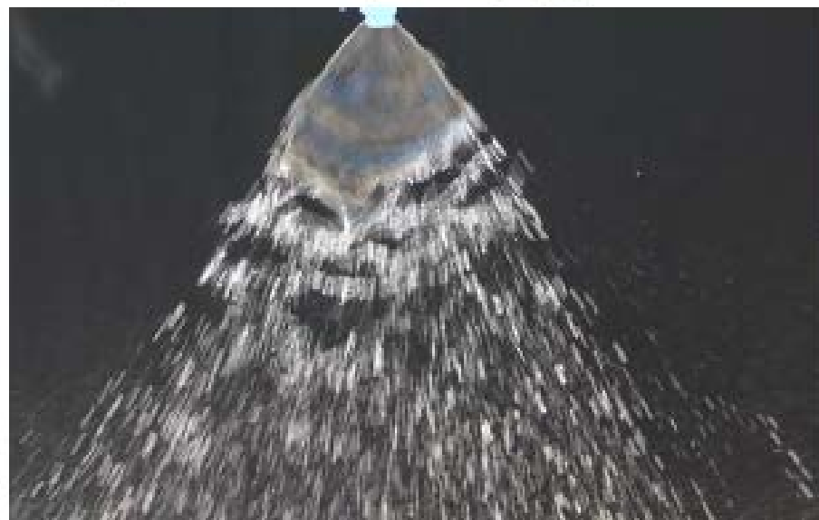
Example of an unacceptable spray pattern
