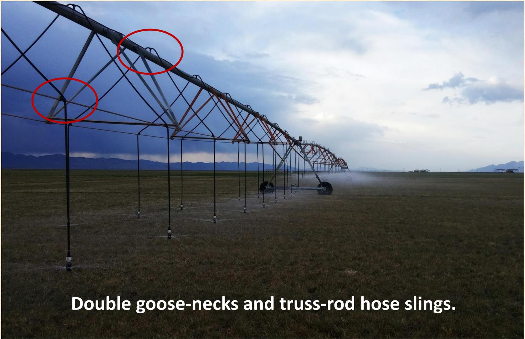
**Double goose-necks and truss-rod hose slings.**
